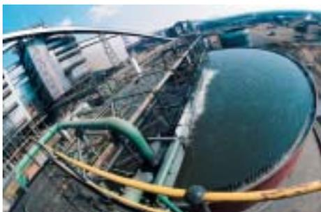
*A thickener tank at the Boshhoek smelter.*
